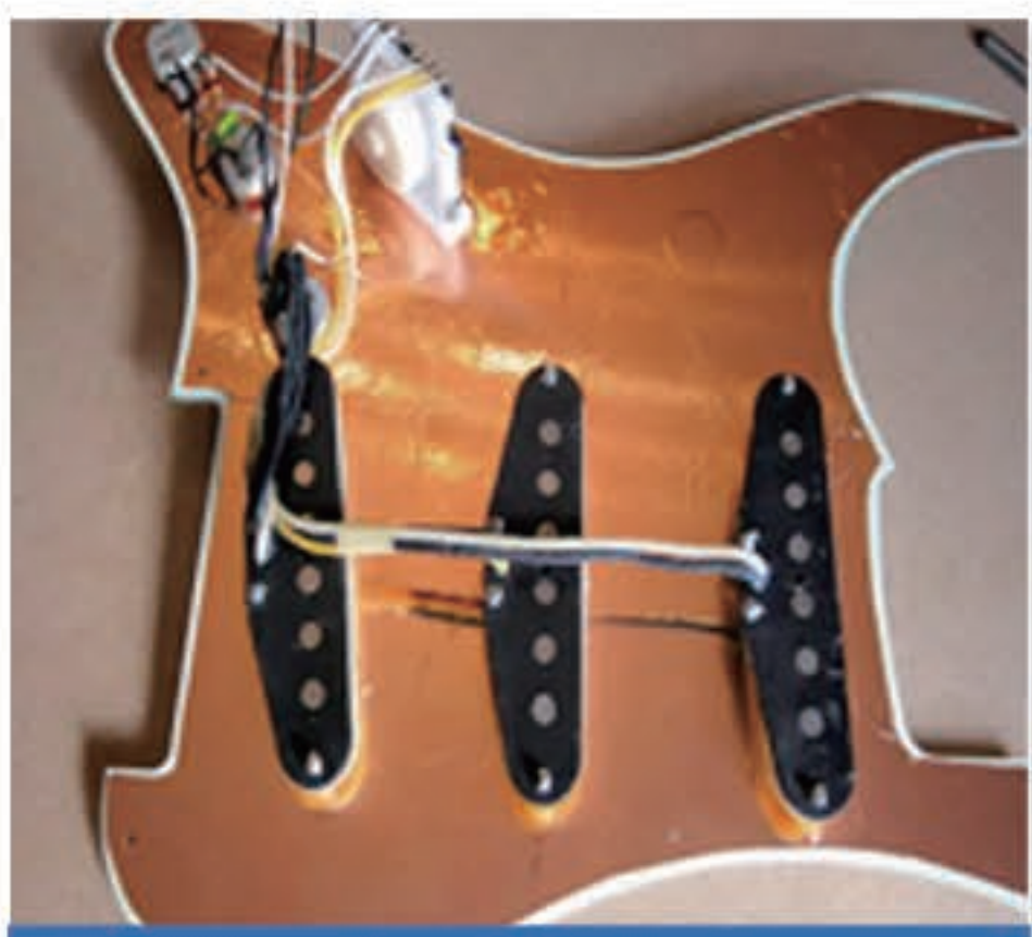
Guitar Circuit Bin Shielding
